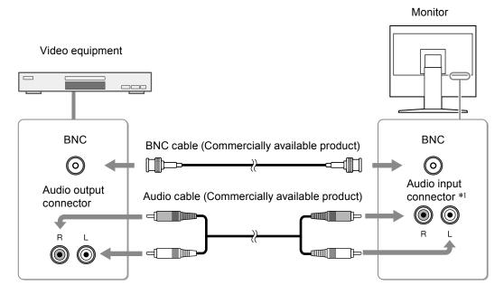
\*1 The monitor is equipped with a single audio input connector to connect for either a PC or visual equipment. Regardless of the input device selected, the monitor will output sound.
